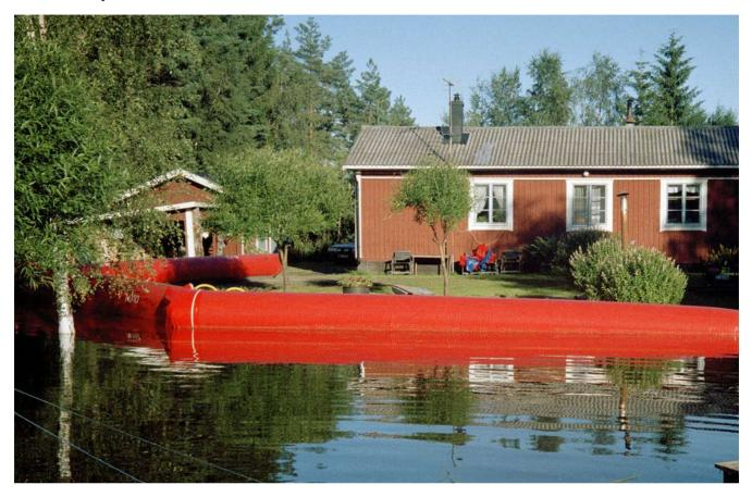
NOAQ Tubewall is a temporary flood barrier. It consists of a number of air inflated sections ("tubes") that are interconnected by ordinary zips to form a continuous protective barrier.
